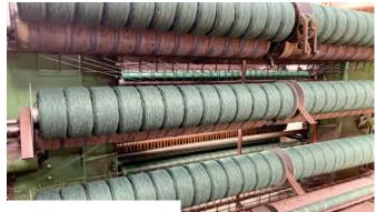
The old machinery which spins recycled fibres into new thread
